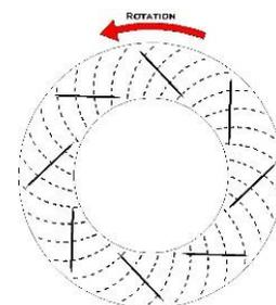
8. The minimum disc thickness is printed on the bell section of the disc. Please note this measurement. Check this measurement before and after track events especially. Do not use the disc beyond this point. Replacement discs for your application are available.
